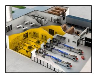
Medium Hygiene Zone contains food and beverage processing with equipment like tanks, vats, vessels, piping, and other storage or transferring apparatus. While there are no open processes in the medium zone, all equipment is flushed, washed, drained, and sanitized. This means industrial panels, enclosures, and accessories must be engineered for easy water runoff or drainage to prevent pooling, as well as interaction with chemicals and cleaning agents without corrosion.
