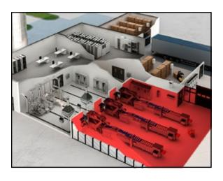
High Hygiene Zone contains a variety of open processes exposed to a variety of surfaces and thus requires the highest degree of sanitation. Industrial panels and enclosures must have the greatest degree of protection against corrosion from cleaning agents and must facilitate runoff to prevent pooling from frequent wash downs. In addition, equipment in the high hygiene zone must be able to withstand elevated degrees of water pressure and water temperature.
