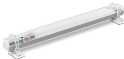
You can use magnets or screws to affix the light holder. The light can swivel in the holder. Connect the supply voltage to the light via Push-in connection. You do not require special connectors for this. You can connect several lights in succession. A button is used to switch the light on and off.
