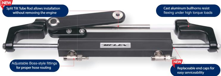
With its revitalized, yet familiar design, the new UC95-OBF cylinder (formerly known as the UC94 OBF) raises the bar for hydraulic steering applicable to engines up to 175 HP. New features of the UC95 include increased horsepower range from 150HP to 175HP, replaceable end caps, and an exclusive split and pinned rod for easy installation.
