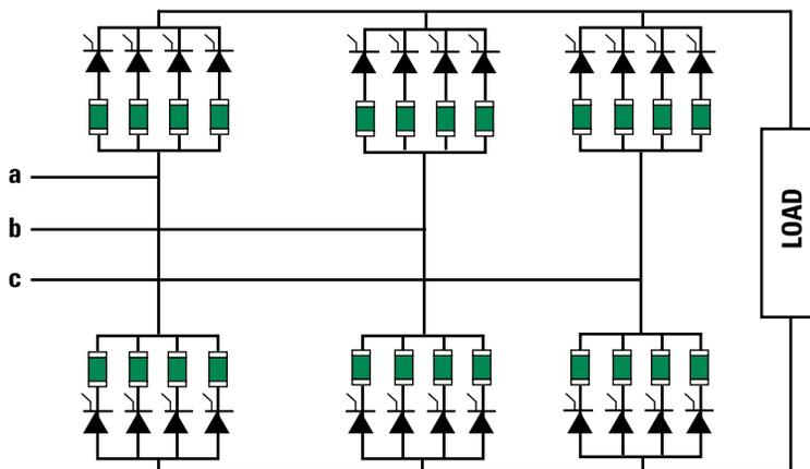
**Figure 29.** Multi-parallel connection in a rectifier circuit
