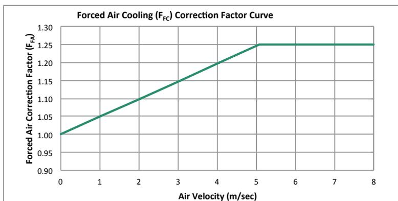
**Figure 30.** Forced (air) cooling correction factor ( $F_{FC}$ ) curve
