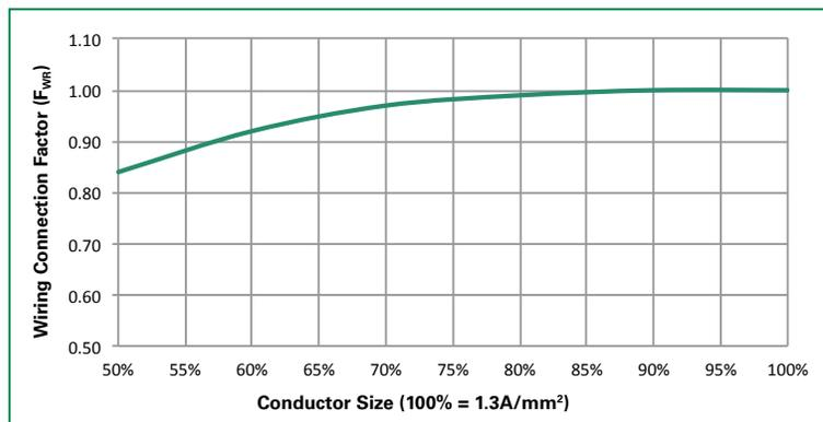
**Figure 31.** Wiring connection factor ( $F_{WR}$ ) curve
