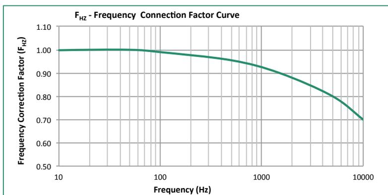
**Figure 32.** Frequency Correction Factor ( $F_{HZ}$ ) Curve
