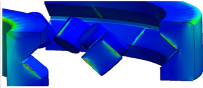
Figure 2. Stress analysis showing how crossed roller bearings can handle radial, thrust and moment loads from any direction at the same time.
